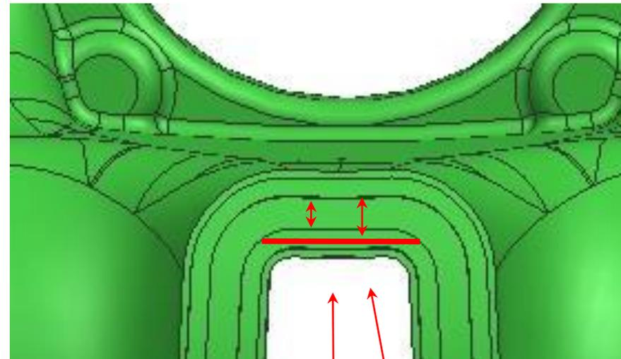
Increase weld bead width from 4mm to 4.5 or 5 mm
