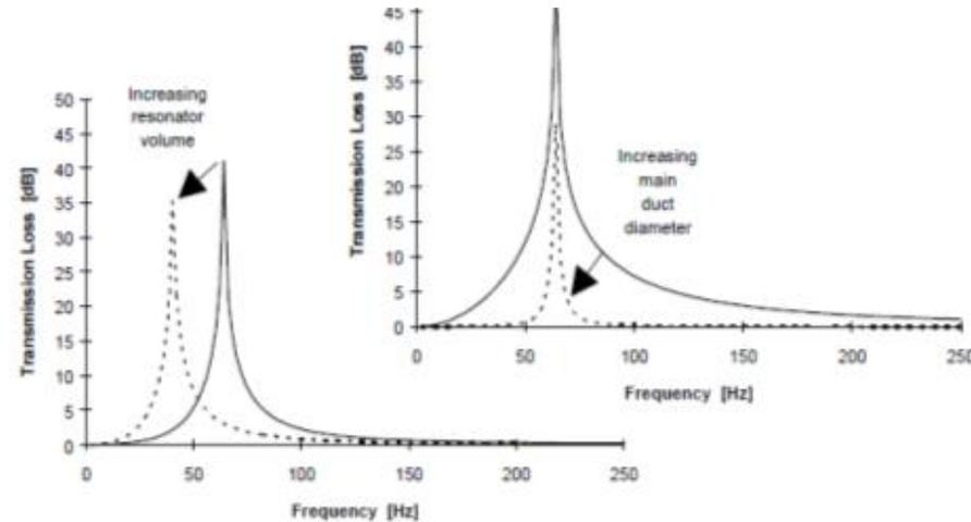
$$\text{Resonant frequency} = f_r = \frac{c}{2p} \sqrt{\frac{S_b}{VLb'}}$$
